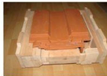
Fig. 5 1 st 3D wooden or resin hard-model of H-cassette for functional test with roofing tile
